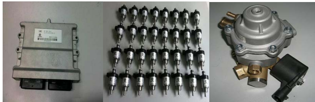
CAERI Engine ECU, Injector and Pressure Regulator
